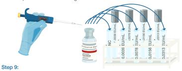
Quickly vortex the content in each tube for a few seconds and immediately place in the Toxinometer® at  $37^{\circ}\text{C} \pm 1^{\circ}\text{C}$  for 60 minutes ( $\pm$  2 minutes). Remember to have laboratory equipment in an area with no vibration.
